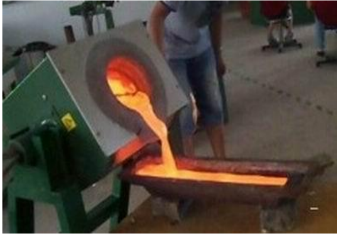
Figura I.45. Horno de inducción DW.MF-160 – Shenzhen, Luohu, China – S.M. Cali Chuen - DaWei Induction Heating Machine Co.Ltd
